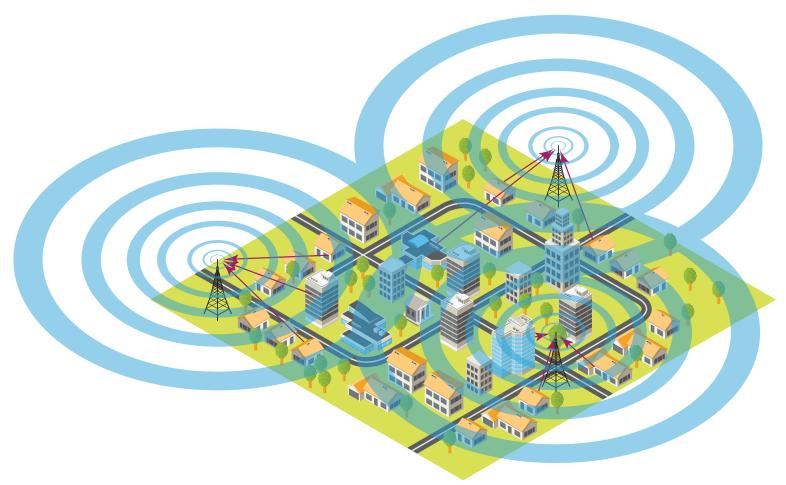
An locast network features licensed narrowband channels and a carrier-grade MAC layer, enabling secure and reliable wide-area communication with mobile and fixed nodes. A base transceiver can cover a single building up to a 1,200 square mile rural area. 4-7 base stations typically cover a major urban center, supporting multiple concurrent applications and millions of nodes. Authorized nodes may securely roam between systems.
